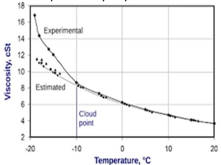
Oil is heated to above the wax appearance temperature. It is then cooled gradually and the viscosity is measured at various temperatures. When the viscosity deviates from a linear increase, the wax appearance temperature (WAT) has been reached.
